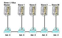
You have to configure a Sinec-L1-bus, own the master, but there's no BT-777-busterminal to buy? No problem, connect the IBX-Klemme to every S5-PLC that is in the run via the optional IBX-SPS-cable, supply every IBX-Klemme with ext. 24V DC if the PLC is not able to provide it, set-up the address 0 and define the actual L1-bus-address in the PLC. Now your master can communicate with the slave-assemblies.
