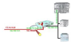
You have in your facility machines from different manufacturers and no one does get access to the controls of the other? No problem, with the S7-firewall you can filter who can ever communicate with the control network and which user with which end users. This is done through the IP address and MAC address.
