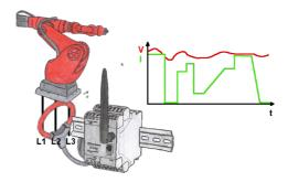
Detect the efficiency of your plant/machine by EtherSens-Energy-devices. Log the preset parameters and evaluate them then later. Find so unnecessary idle-times and increase so the efficiency.
