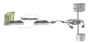
You have to reach urgend your PLC via remote maintenance and have no TS-adaptor in your company? No problem, configure with the MPI-Kabelmanager your S7-interface-cable MPI/PPI-Kabel the mode "TS" for "remote maintenance", connect this cable with the TS-Adapter (article number 9350-TS) with a standard modem and send it all to your client. Now you will be able to start the connection with your TS-sofware and solve the problem. And this all without buying a original TS-adapter.
