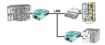
Your pumping stations report the water levels of the central control via telephone network. The central office itself can of course transmit commands/messages to the substations as well. Thereto no dedicated line is required, it's sufficient when the stations connect via network (DSL-router).
