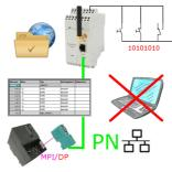
Via digital input triggered DB-backup/-restore without additional PC via MPI/Profibus to FTP-server
