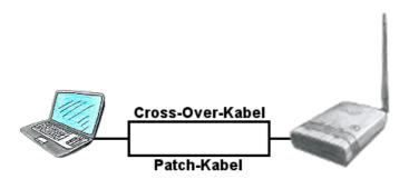
You need ALF to connect to a reachable WLAN, but only have a patch-cable? No problem, ALF provides "autonegotiation" and this means that he recognises a connected cable (patch-cable or cross-over-cable) and surround the pinning according to the cable, so a communication is possible.
