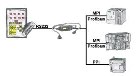
Your panel provides a serial port and no MPI/Profibus for connecting a S7-PLC. Connect the MPI-II-cable with it and you're Online with your panel.
