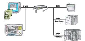
Your panel only has a LAN-socket as PLC-interface? No problem, connect this socket with the S7-LAN or the MPI-LAN-cable and plug it directly on the PPI/MPI/Profibus of the PLC. Then access to the variables and data of the PLC is already available.
