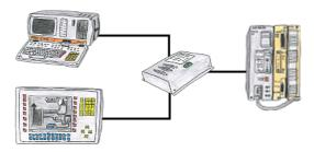
Your PD-interface of the S5-PLC is already occupied with a panel and you should accomplish program modifications without removing the panel? No problem, connect the Multiplexer one-time to the PLC and then connect the panel and also your PC to the Multiplexer. Now you can work parallel with the PLC without the need of affecting the operation of the panel.
