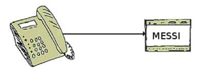
The MESSI remote-station will be called directly by integrated mobile-phone. If a connection comes off, digital In- and Outputs for teleswitching will be transmitted. Each device can both transmit state of things and accordingly receive switch signals.
