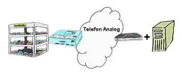
Your car park or control sends the configuration/capacity utilisation to a PC with a modem, so that the data can be used for further processing.
