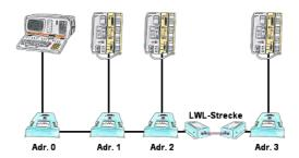
You need for your L1-Bus higher distance like the possible 1200m? You have strong distrubance on your L1-Bus? You need a serial line for higher distances and this galvanic decoupled? No problem, all this points are solved through the LWL-adapter. They are available for artificial and optical fibre, for L1-Bus and RS232.
