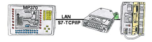
Your panel only has a LAN-socket as PLC-interface and supports only S7-RFC1006, no problem. Connect this socket with the S5-LAN++ and plug it directly on the PD-interface of the PLC. The S5-LAN++ performs adverse your panel as a S7-PLC although you receive the data from the S5-PLC. Then access to the variables and data of the S5-PLC is already available.
