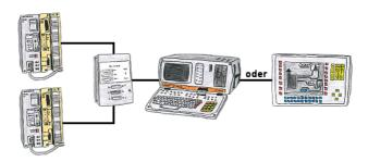
You have to work with more PLC-devices, but no pleasure to switch on/off? No problem, you connect a device of the AG-Switch-family to the PLC-devices and your PD/PC and you will be able to communicate to both PLCs. The selection which PLC you make for AG-Switch-I via toggle switch and for the AG-Switch-II via 24V-controll input.
