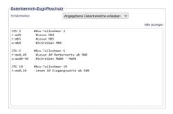
With the management of the data-areas it is determined whether the entered data-areas can be read/written via the module with the connected controllers. A central button for the function determines whether the specified inputs are "allowed" or "not allowed" are.
