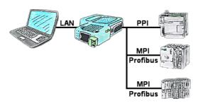
S7-PLC with PPI, MPI, Profibus connection, but data should be read/written via network?
