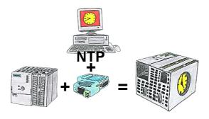
You need in your PLC a actual time? No problem, with the NTP-function the S7-LAN-module get from a NTP-(Time-)Server the actual time and transfers it direct into the configured PLC or for processing in a DB.
