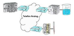
Your pumping stations report the water levels of the central control via telephone network. The central office itself can of course transmit commands/messages to the substations as well. Thereto no dedicated line is required, a "normal" telephone connection is sufficient because the devices hangs up the line after occured message.
