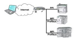
You have access to a on-site network and your PLC-device has no LAN-connection? No problem, plug the S7-LAN on the PLC-device and you will have immediate access to the PLC from afar.
