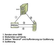
A SMS to a mobile phone is basically send by SMSC. Within the GSM-network it takes place via on-net SMSC. Thereby it's unimportant in which mobile network the receiver is. The message is activated by:
