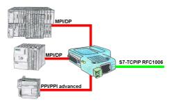
Networking of all S7-controllers (S7-200/300/400), for example with your production-data-acquisition, Industry 4.0 (OPC Server UA or Classic), panels and other devices that communicate via S7-TCPIP RFC1006. One module for all bus-types: PPI, MPI and Profibus.
