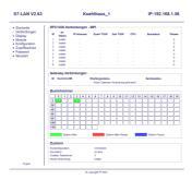
View information from the connected bus-system in plain text without using the Simatic-Manager or TIA-Portal. With the connection-menu you get the list of reachable nodes, marked in color whether it is an "active bus-participant", is a "candidate for inclusion in the bus" or a "passive bus-participant".
